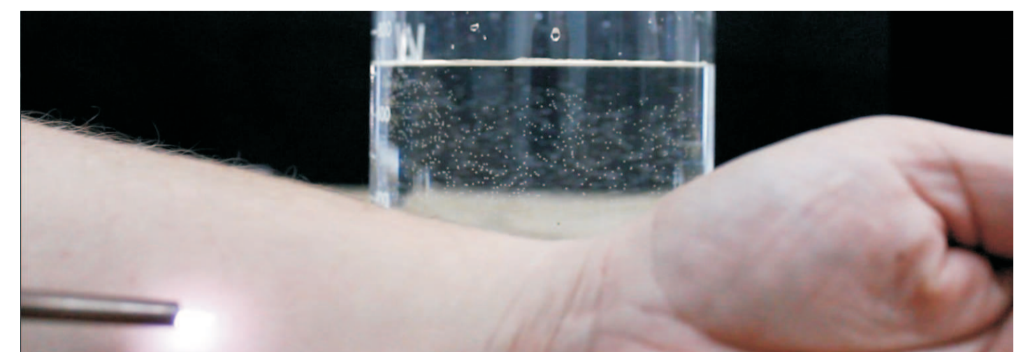
Photo of the low power Ar microplasma treatment of the human skin
